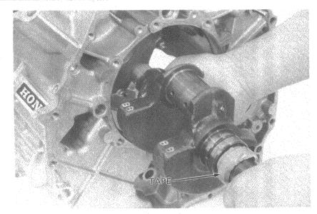
Install the O-ring and collar. Install the crankshaft holder cap. Install the guide bolts in the crankshaft holder cap as shown.
