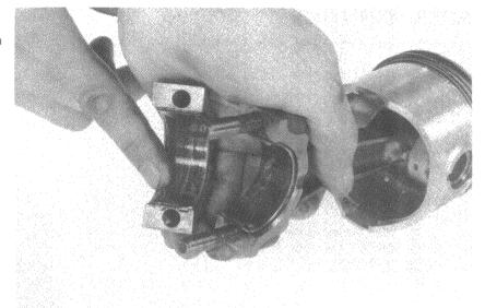
Install the rod assemblies into the cylinders from the top of the engine case.
