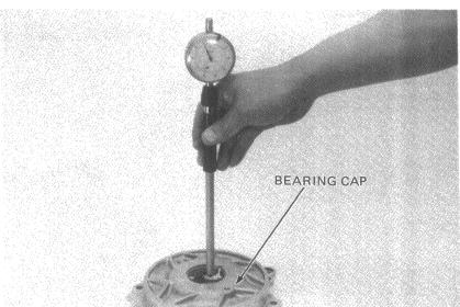
If rod bearing clearance is beyond tolerance, select replacement bearings as follows.
