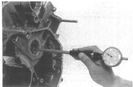
Measure the crankshaft cap bearing support I.D.
