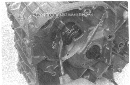
Turn the crankshaft so that the piston is at T.D.C.
