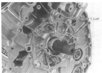
Attach the CRANK CAP PULLER to the front of the engine.
