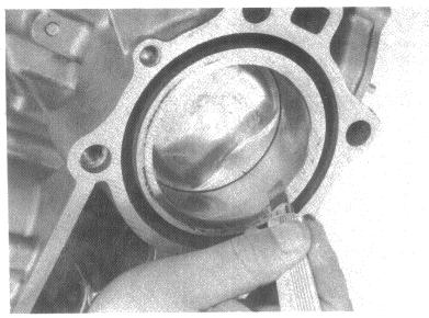
Turn the crankshaft so that the piston to be removed is at B.D.C. (Bottom Dead Center). Remove the bearing cap.
