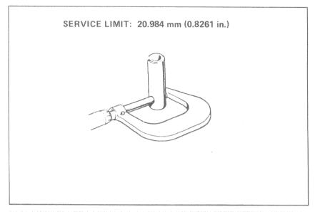
Measure the rod end I.D. If the reading exceeds the service limit, replace the rod.
