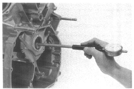
Measure the engine case and crankshaft bearing cap I.D.
