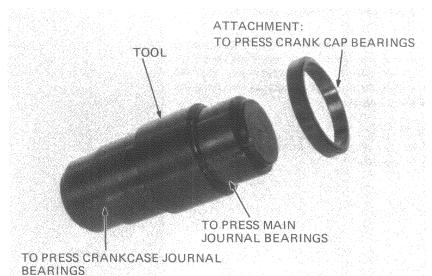
Press the bearings out of the crankshaft cap bearing support with a hydraulic press and bearing removal tool.
