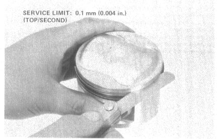
Insert each piston ring into the cylinder and measure the ring end gap.
