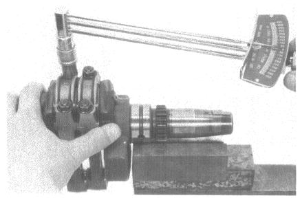
Remove the caps and measure the compressed plastigauge.
